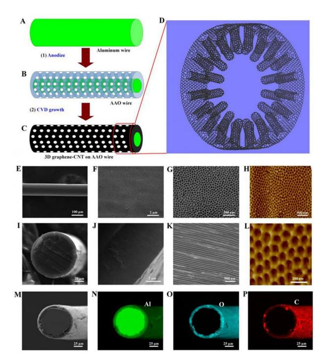
Schematic diagrams showing the synthesis and microstructures of a 3D graphene-RACNT fiber. (A) Aluminum wire. (B) Surface anodized aluminum wire (AAO wire). (C) 3D graphene-RACNT structure on the AAO wire. (D) Schematic representation of the pure 3D graphene-RACNT structure. (E to G) Top view SEM images of the 3D graphene-RACNT fiber at different magnifications. (I to
