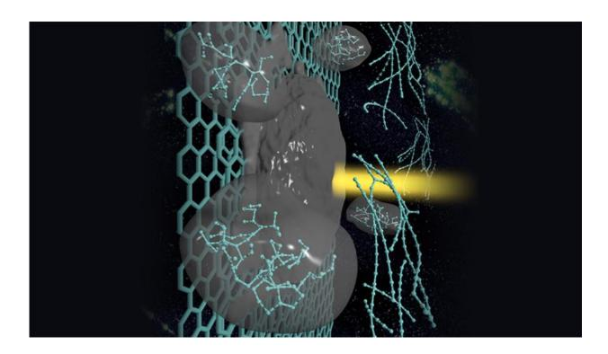
A carbyne strand forms in laser-melted graphite. Carbyne is found in astrophysical bodies and has the potential to be used in nanoelectronic devices and superhard materials. Credit: Liam Krauss/LLNL
