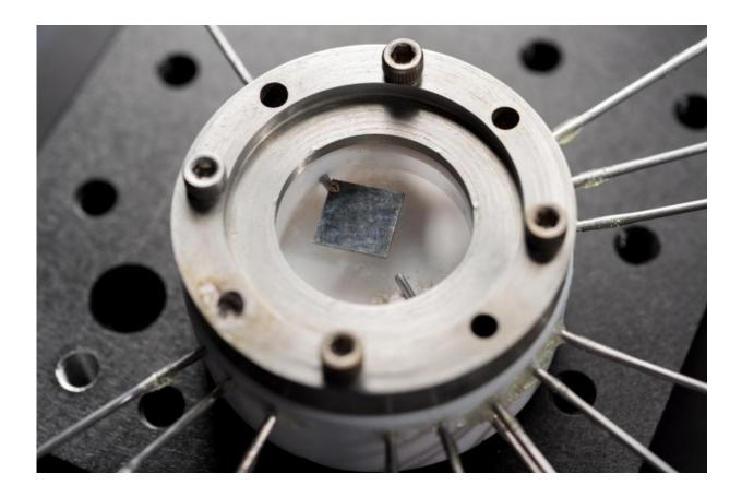
Shown is a sample holder used to test samples of lithiated silicon to determine its nano-mechanical properties. The device was used to develop a detailed nano-mechanical study of mechanical degradation processes in silicon thin films. Credit: Rob Felt, Georgia Tech
