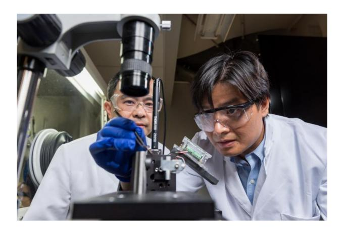
Professor Ting Zhu and Assistant Professor Suman Xia, both from Georgia Tech's Woodruff School of Mechanical Engineering, show how a thin film electrode made of amorphous silicon was tested in a custom environmental indenter. To provide proper environmental control, samples containing lithiated silicon were tested with the device inside the glove box shown in the background. Credit: Rob Felt, Georgia Tech
