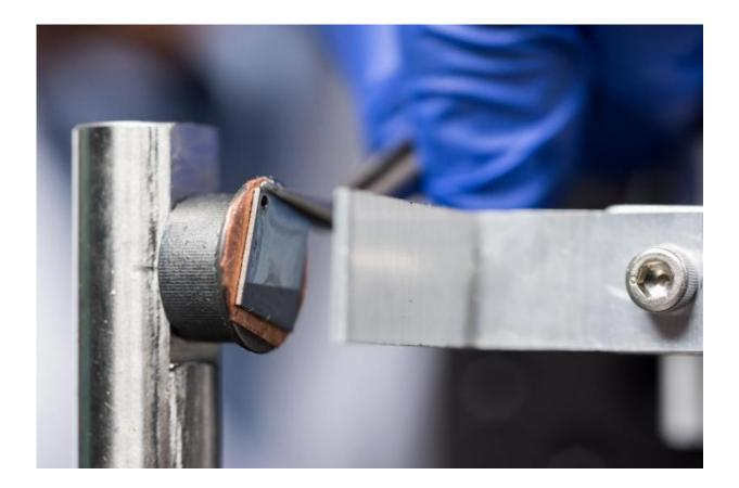
Shown are details of a custom environmental indenter used to test thin film electrodes made of amorphous silicon. The device was used to develop a detailed nano-mechanical study of mechanical degradation processes in silicon thin films. Credit: Rob Felt, Georgia Tech
