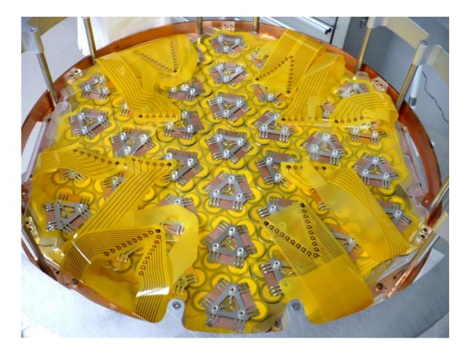
Part of the EXO-200 underground detector used to search for a hypothesized radioactive decay that could reveal how neutrinos acquire their incredibly small mass. Credit: EXO Collaboration
