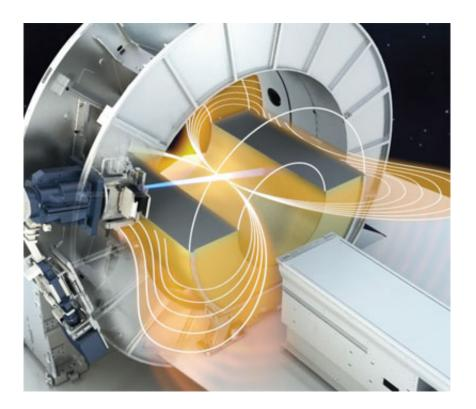
Representation of an MRI linear accelerator, a proposed system for radiotherapy treatment. Credit: Elekta
