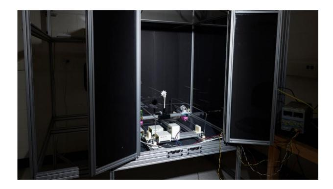
The test chamber used to study hawkmoths includes a robotic flower that can be moved with positioning equipment taken from a 3-D printer. Infrared video cameras track the movement of the insects, which normally fly only during low-light conditions. Information from the research could help future generations of small flying robots deal with challenging computational and vision requirements.
