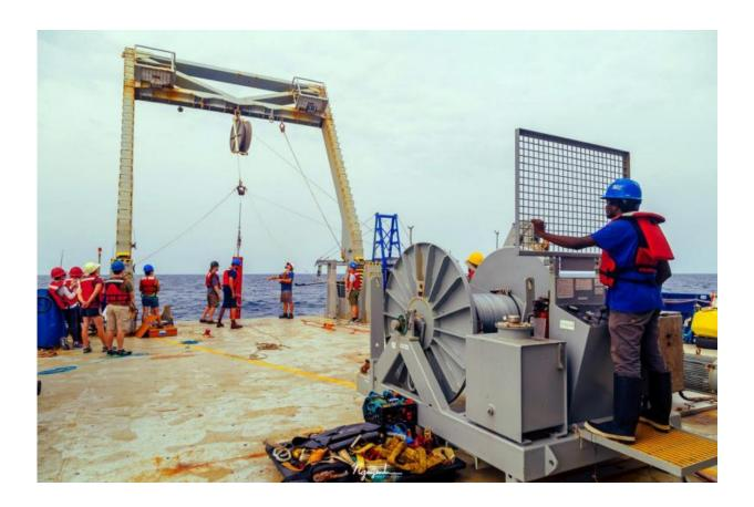
US and Indian scientists aboard the research vessel R/V Roger Revelle deploy a drifting spar buoy to measure upper ocean density and velocity in the Bay of Bengal. The month-long, ONR-sponsored mission centered on monsoon prediction. Credit: the R/V Roger Revelle
