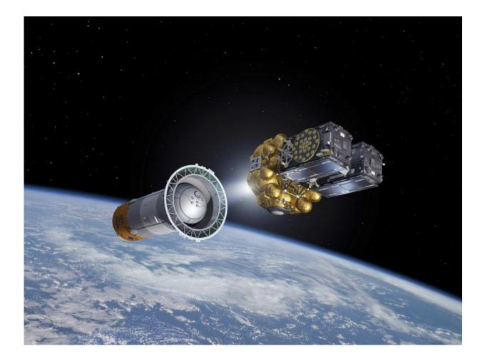
Artist's view of Galileo satellites attached to their dispenser atop their Fregat upper stage separating from the Soyuz upper stage. The Fregat then flies them the rest of the way up to medium-Earth orbit. Credit: ESA–J. Huart, 2014
