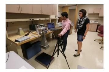
Ali Foudazi adjusts an infrared thermograph as the horn microwave heats up a section of concrete to test for flaws. Kristen Donnell, right, has been studying
