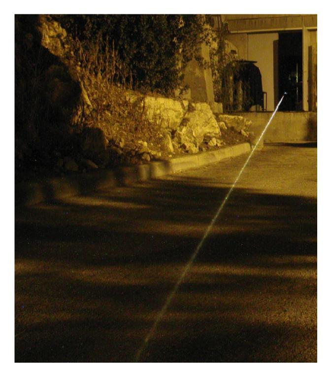
A picture of a femtosecond laser. The laser beam itself is invisible (800nm), but due to the formation of a plasma channel, the beam emits (visible) white light. Credit: Jenya Papeer, Hebrew University, Israel
