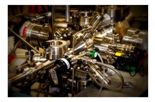
The team uses a Scanning Tunnelling Microscope (STM) to inject atoms onto a surface in a precise pattern, enabling them to build nanoscale devices more quickly and easily than before
