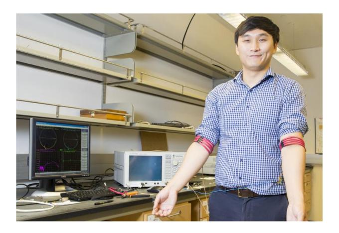
Jiwoong Park, an electrical engineering Ph.D. student and first author of the study, demonstrates communication from arm to arm using the magnetic field human body communication prototype developed in Mercier's Energy-Efficient Microsystems Lab at UC San Diego
