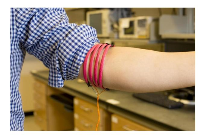
A prototype of the magnetic field human body communication, developed in Mercier's Energy-Efficient Microsystems Lab at UC San Diego, consists of magnetic-field-generating coils wrapped around three parts of the body, including the head, arm and leg. Credit: Jacobs School of Engineering, UC San Diego
