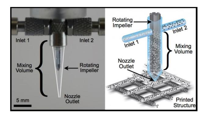
An Impeller-based active mixer. Each fluid enters the mixing chamber through a separate inlet and is mixed in a narrow gap by an impeller rotating at a constant rate. Credit: Thomas Ober, Harvard SEAS/Wyss Institute
