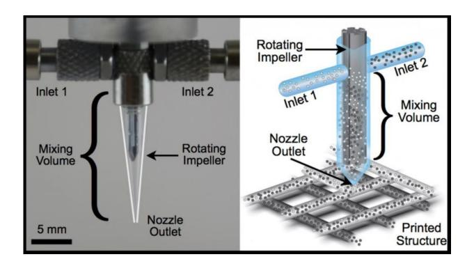
An Impeller-based active mixer. Each fluid enters the mixing chamber through a separate inlet and is mixed in a narrow gap by an impeller rotating at a constant rate. Credit: Thomas Ober, Harvard SEAS/Wyss Institute
