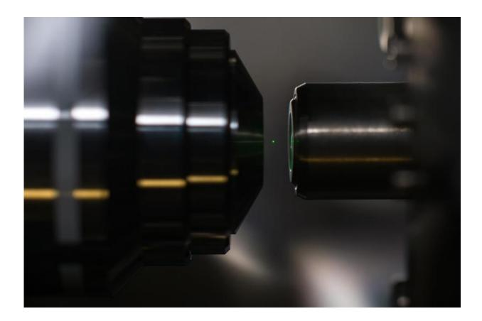
A nanodiamond containing hundreds of nitrogen vacancies glows while levitated by a laser during an experiment in Nick Vamivakas' lab at the University of Rochester. The team have now continued the research to use nanodiamonds with single vacancies and to do the experiments in vacuum. Credit: J. Adam Fenster/University of Rochester.
