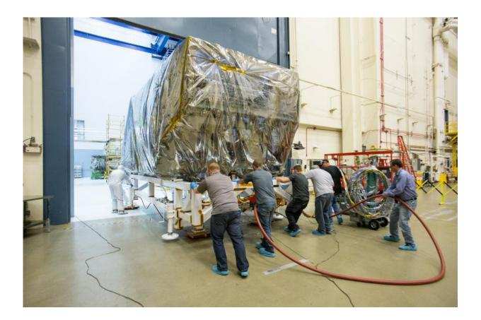
The wrapped up ISIM structure pushed back to the clean room post acousticstest, to prepare for the EMI test. Credit: NASA/Desiree Stover
