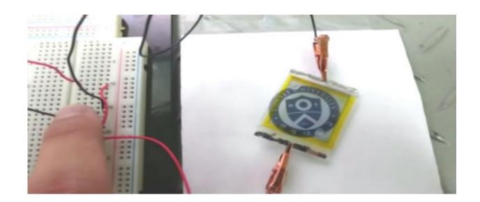
Scientists have developed a new hybrid, solar-energy system that harnesses the full spectrum of the sun's radiation by pairing a photovoltaic cell with polymer films. The films convert the light that goes unused by the solar cell into heat and then converts the heat into electricity. They report on their device, which produces a voltage more than five times higher than other hybrid systems, in the journal *ACS Nano*.
