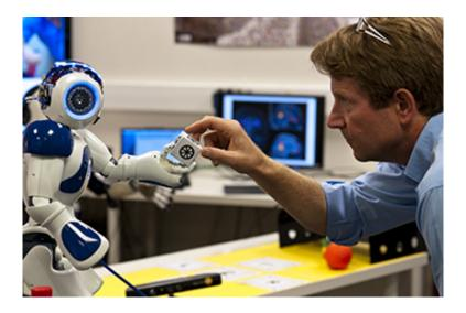
Peter Ford Dominey and the robot Nao, study of developmental robotic cognition. Instead of using pre-established plans, the robot can learn in real time through direct interaction with a human. Credit: © Inserm/Patrice Latron
