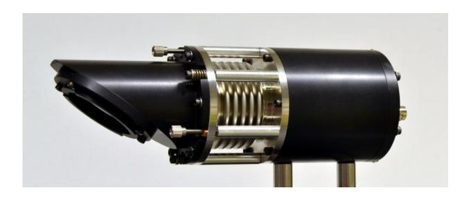
PQED consists of a Brewster window (left) protecting the detector elements from impurities, adjustable bellows and the detector chamber itself. In order to further decrease uncertainties in measurement, the window was removed and the detector was protected from impurities using nitrogen flow.
