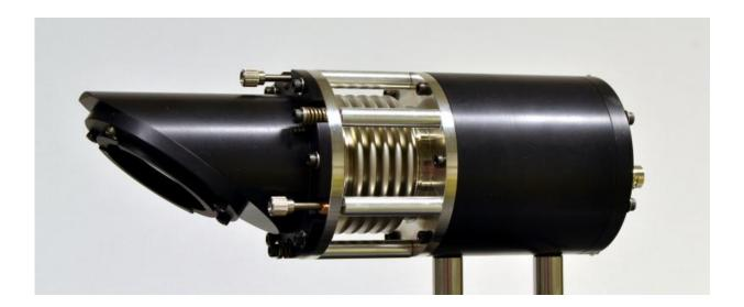
PQED consists of a Brewster window (left) protecting the detector elements from impurities, adjustable bellows and the detector chamber itself. In order to further decrease uncertainties in measurement, the window was removed and the detector was protected from impurities using nitrogen flow.
