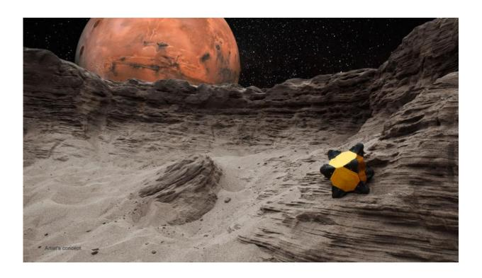
While a Mars rover can't operate upside down, the Hedgehog robot can function regardless of which side lands up. Credit: NASA/JPL-Caltech/Stanford
