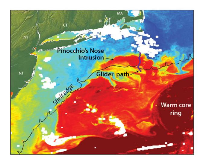
Satellite imagery shows the exchange of warm core ring water (red) with the colder continental shelf waters (blue). Satellite imagery, however, could not help scientists determine the underlying process for the warm water intrusion; instead they used data from ocean robots or "gliders" recently installed off the coast of Massachusetts. The scientists have dubbed the events "Pinocchio's Nose
