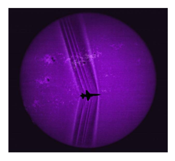
Using the solar disk as a backdrop, its details revealed by a calcium-K optical filter, researchers processed this image to reveal shock waves created by a supersonic T-38C. Credit: NASA Photo
