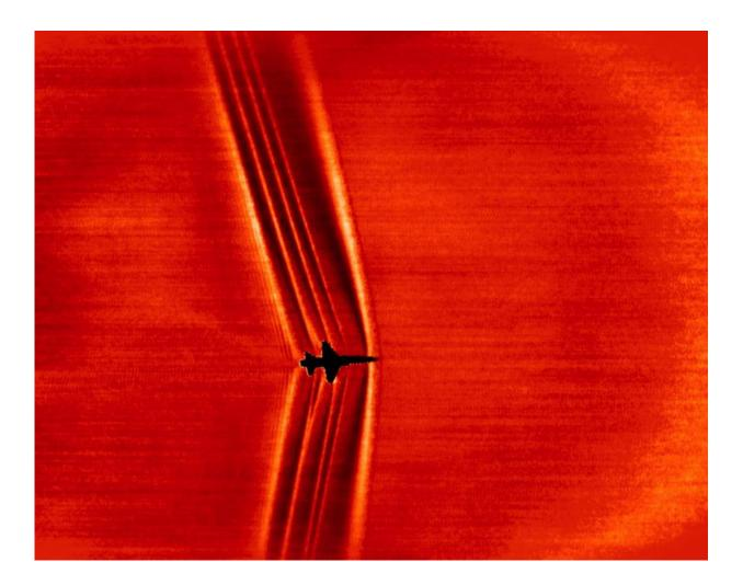
This schlieren image of a T-38C was captured using the patent-pending BOSCO technique and then processed with NASA-developed code to reveal shock wave structures. Credit: NASA image
