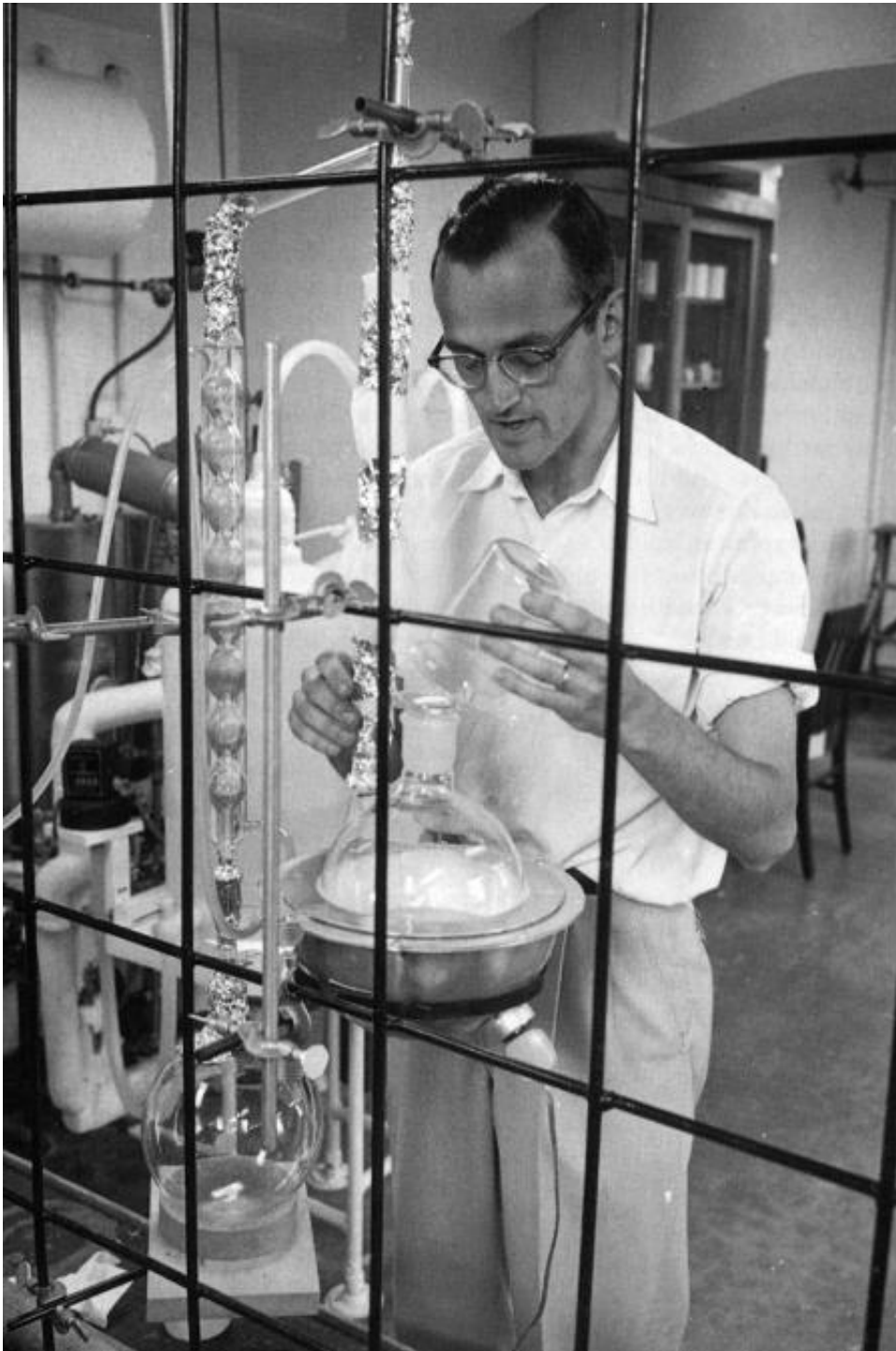
In his sleuthing for trace amounts of lead, Caltech geochemist Clair Patterson redistills a reagent in this 1957 photograph. He didn't trust the purity of commercial chemicals. Credit: Caltech E&S Magazine, Volume 60, Number 1, 1997
