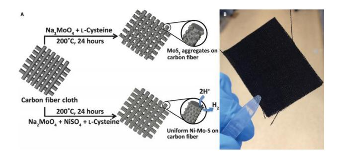
Synthesis processes of MoS2/C and Ni-Mo-S/C. (A) Schematic illustration of syntheses of MoS2 and Ni-Mo-S on carbon fiber cloth. (B) Photographic image of freshly prepared Ni-Mo-S/C (1:1). Credit: *Science Advances*, DOI: 10.1126/sciadv.1500259
