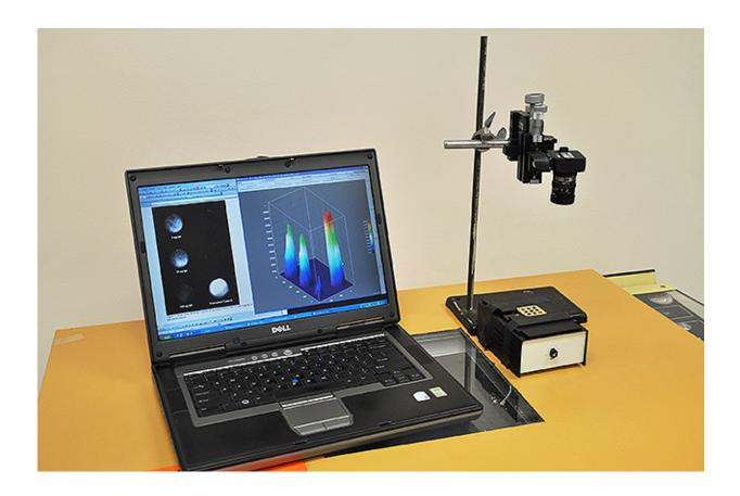
ARS scientists have developed this low-cost apparatus for detecting active Shiga toxin. Credit: Reuven Rasooly
