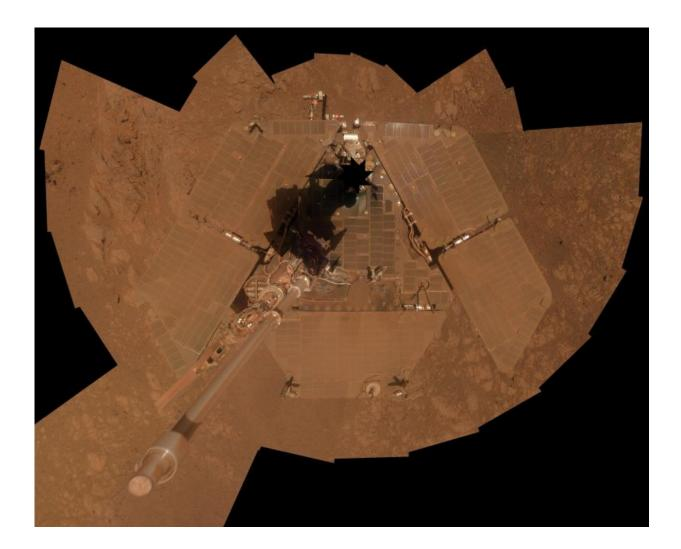
A dust storm on Mars in 2008 temporarily cuts the amount of sunlight reaching the solar array on NASA's Mars Exploration Rover Spirit, leaving the rover in a
