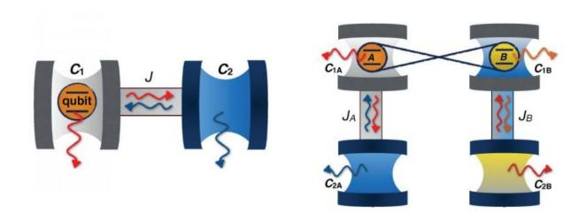
(Left) In the single-qubit system, a qubit is embedded in a cavity, which in turn is coupled to a second cavity by a coupling strength J. (Right) In the two-qubit system, two entangled qubits are each embedded in their own cavity, and each cavity is coupled to a second cavity. Credit: Man, et al. ©2015 Nature *Scientific Reports*
