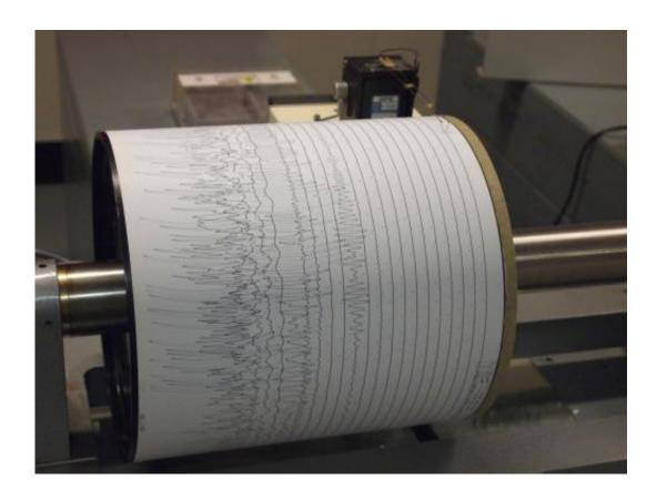
Seismogram being recorded by a seismograph at the Weston Observatory in Massachusetts, USA. Credit: Wikipedia
