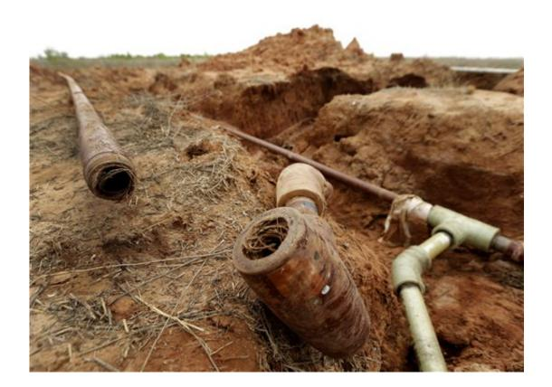
In this April 22, 2015 photo, a saltwater disposal pipe that ruptured lies beside a new pipe on land owned by Wesley Graves near Snyder, Texas. Equipment failure is a major cause of spills of oilfield wastewater. (AP Photo/Charlie Riedel)
