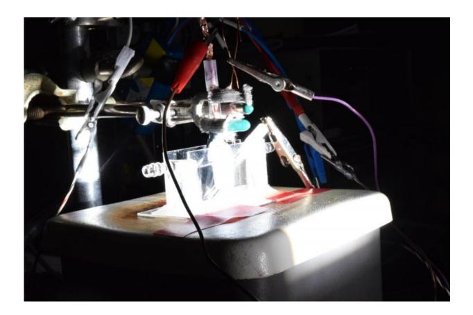
Bathed in simulated sunlight, this photoelectrolysis cell in the lab of Song Jin, a professor of chemistry at the University of Wisconsin-Madison, splits water into hydrogen and oxygen using a catalyst made of the abundant elements cobalt, phosphorus and sulfur. Credit: David Tenenbaum/University of Wisconsin-Madison
