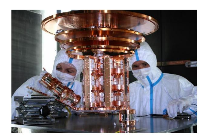
By carefully re-engineering a detector for heavy dark matter particles, so-called WIMPS, the CRESST collaboration succeeded in improving the detector to measure lightweight dark matter particles with masses in the range of a proton mass. Credit: Max Planck Institute for Physics
