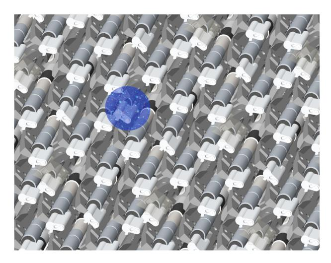
A few of the 5,000 close-packed robotic positioners that place the ends of optical fibers to collect the light from a single galaxy or quasar. The blue circle represents a patch of sky with numerous astronomical targets reachable by a single robot. In seconds it can rotate, extend, or retract to place its fiber in position with millionths of a meter precision. Credit: R. Lafever, DESI Collaboration
