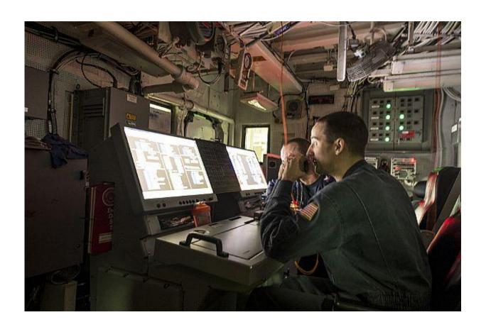
Sailors monitor ship propulsion and fuel levels in an enclosed operating station aboard the amphibious dock landing ship USS Harpers Ferry (LSD 49). The Office of Naval Research is developing cyber protections for shipboard mechanical systems like this. Credit: (US Navy photo by Mass Communication Specialist 3rd Class Mark El-Rayes/Released)
