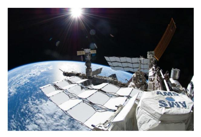
The Alpha Magnetic Spectrometer mounted on the International Space Station could help detect the signs of dark matter. Credit: NASA
