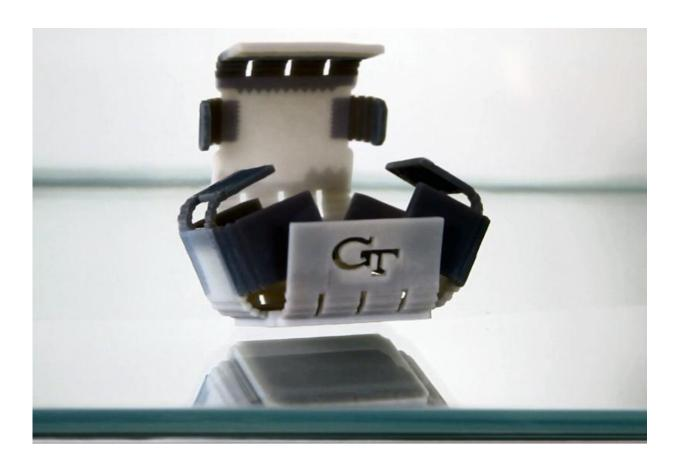
Self-folding process of smart shape-memory materials with slightly different responses to heat. Using materials that fold at slightly different rates is important to ensure that the components do not interfere with one another during the process. Credit: Qi Laboratory, Georgia Tech
