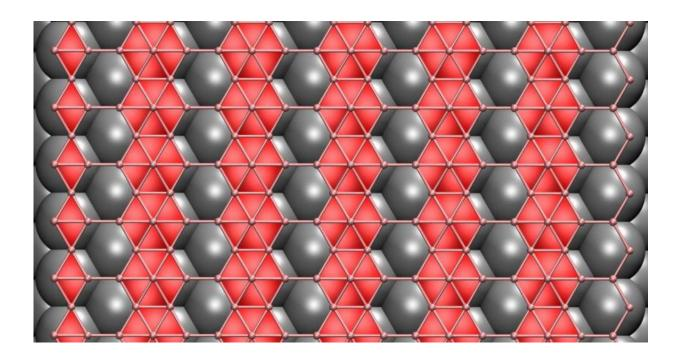
Rice University scientists have determined that still-theoretical two-dimensional boron would adjust its form depending on the substrate used in the growth process. They found that a copper substrate would be best for growing flat boron in a chemical vapor deposition furnace. Credit: Zhuzha Zhang/Rice University
