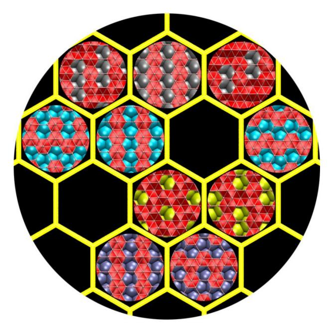
Two-dimensional boron would take a different forms, depending on the substrate used in chemical vapor deposition growth, according to Rice University researchers. Credit: Zhuzha Zhang/Rice University
