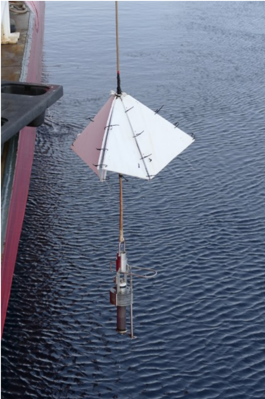
Core on its way up to the Healy. Note the core-of-silence rigged by Tim Kenna and Marty Fleicher to stop any interference with the rosette altimeter used to lower the device. Credit: Bill Schmoker
