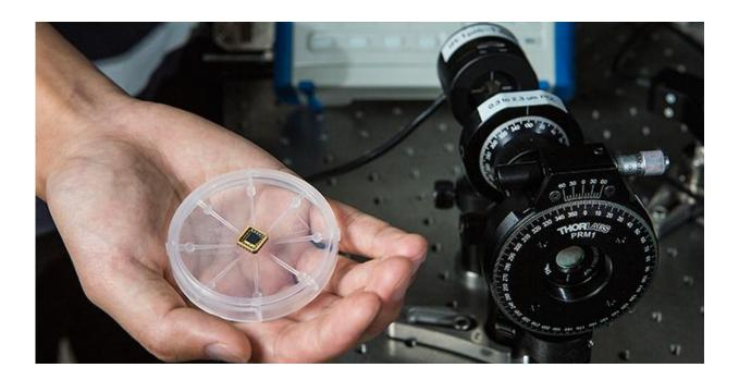
The circularly polarized light detector on a chip, on the left, performs the same function as the conventional, optically based detector on the right. Credit: Anne Rayner, Vanderbilt University
