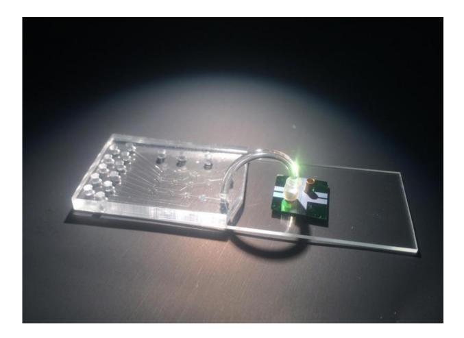
This hybrid device integrates a microfluidic chip for sample preparation and an optofluidic chip for optical detection of individual molecules of viral RNA. Credit: Joshua Parks
