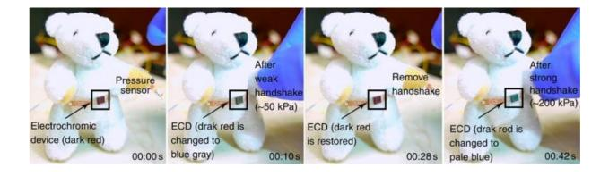
When attached to a teddy bear, the e-skin changes color upon a handshake, since the pressure-sensitive polymer is attached to the paw. Credit: Chou, et al. ©2015 Macmillan Publishers Limited
