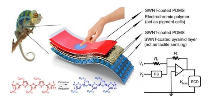
The chameleon-inspired e-skin's two main components are a pressure-sensitive polymer ("pyramid layer") and an electrochromic polymer. At bottom left, the two chemical structures of the electrochromic polymer are shown that emit red and blue light, respectively. (Ambanja panther chameleon and hand images from 123rf.com) Credit: Chou, et al. ©2015 Macmillan Publishers Limited
