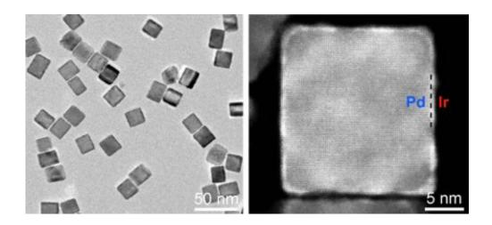
A new catalyst that improves the sensitivity of the standard PSA test more than 100-fold, pictured above, is made of palladium nanocubes coated with iridium.
