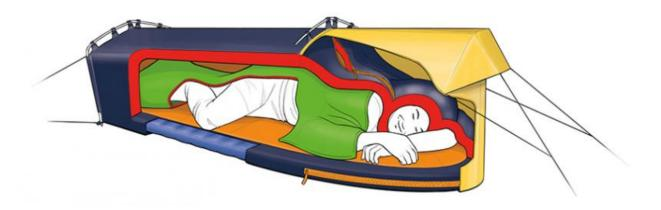
Sleeping cell shell (dark blue) with the zippered air opening and liner (green). Credit: Polarmond
