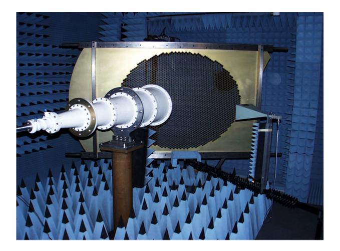
Factory acceptance test of the M6 S/X-band dichroic mirror installed at New Norcia station, Australia (DSA1). Credit: ESA/Telecom Italia
