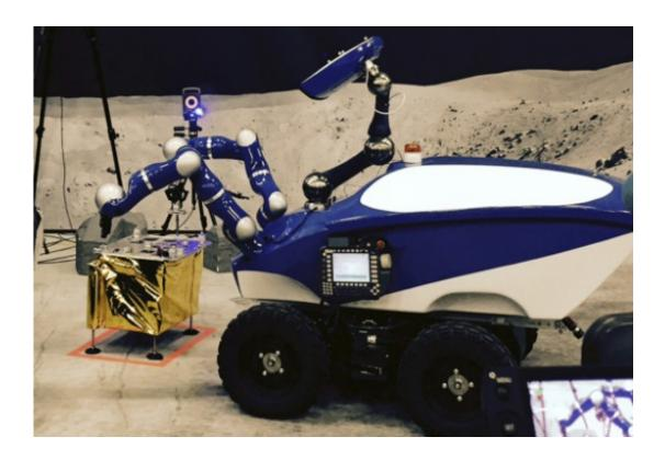
The blue-and-white Interact Centaur fibreglass robot, which cost less than 200,000 euros (\$224,000) to build, has a camera on its head which allows the controller to directly see the task it is performing
