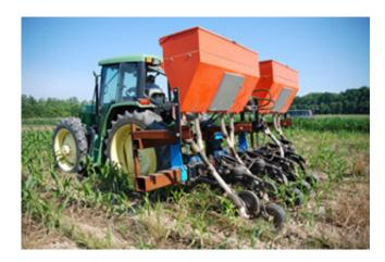
Pelletized poultry litter was applied using a prototype subsurface band applicator
