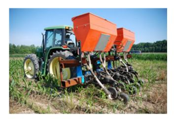
Pelletized poultry litter was applied using a prototype subsurface band applicator
