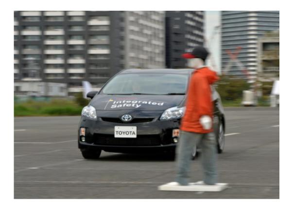
This photo taken on October 10, 2013 shows Japanese auto giant Toyota Motor demonstrating its "pre-collision system" which uses automatic steering in addition to automatic braking to prevent collisions, in Tokyo
