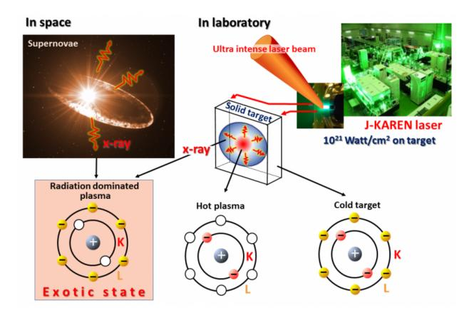
Generation of exotic states – Hollow multicharged ions by ultraintense X-ray photo pumping in space (Supernova explosions) and laboratory (ultra-intense visible femtosecond lasers). (Upper right) A photo of J-KAREN, KPSI and JAEA's high power laser facility. Credit: Osaka University
