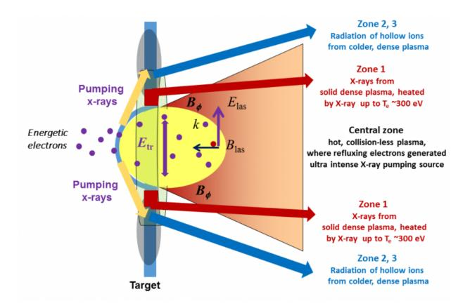
Scheme of ultra-intense x-ray source generation in relativistic laser-produced plasma. The strong x-rays generated in the Central Zone illuminate the periphery which the laser does not hit (Zone 1~3). Credit Osaka University
