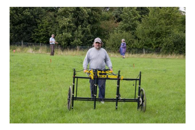
A four-sensor magnetometer in action at Verulamium. Credit: Kris Lockyear
