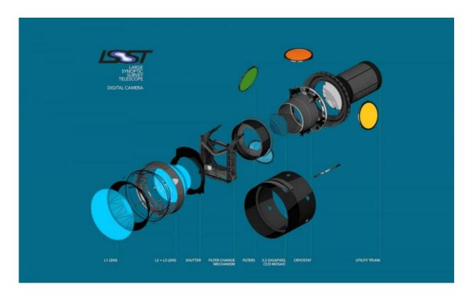
This exploded view of the LSST's digital camera highlights its various components, including lenses, shutter and filters. Credit: SLAC National Accelerator Laboratory
