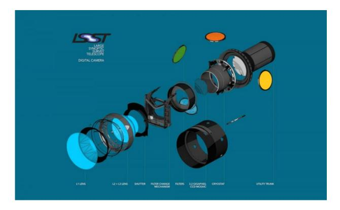
This exploded view of the LSST's digital camera highlights its various components, including lenses, shutter and filters. Credit: SLAC National Accelerator Laboratory
