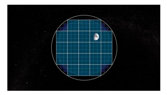
In one shot, the Large Synoptic Survey Telescope's 3.2-gigapixel camera will capture an area of the sky 40 times the size of the full moon (or almost 10 square degrees of sky). LSST's large mirror and large field of view work together to deliver more light from faint astronomical objects than any optical telescope in the world. Credit: SLAC National Accelerator Laboratory
