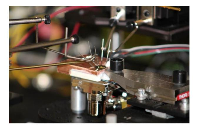
A photonic integrated circuit (PIC) used to cancel radio-frequency interference being tested on an optical probe station. Probes provide electrical contact while a fiber launch stage measures output light from the PIC. The PIC is 2.5 mm x 1 mm in size. Credit: Paul Prucnal, Department of Electrical Engineering, Princeton University
