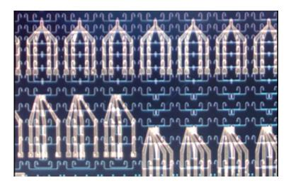
A silicon photonics platform used to support interconnections among excitable lasers and forming a photonic neural network on-chip. Credit: Paul Prucnal, Department of Electrical Engineering, Princeton University
