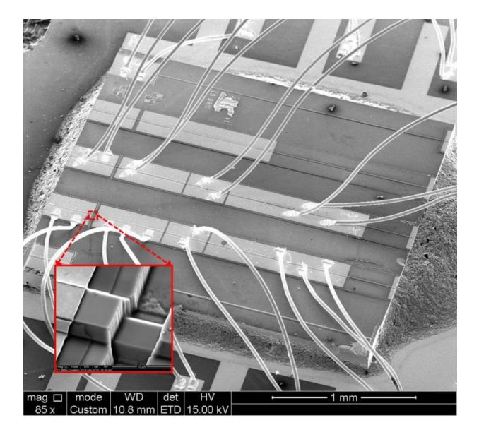
A Scanning Electron Microscope image of a photonic integrated circuit designed to cancel radio-frequency interference. The inset shows an etched facet used for a monolithic Fabry-Perot laser. The right hand plots show the photonic integrated circuit reducing and eliminating interference. Credit: Paul Prucnal, Department of Electrical Engineering, Princeton University
