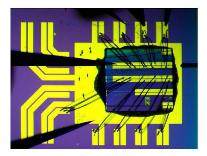
An optical microscope image of the PIC. This chip provides wide bandwidth radio-frequency interference cancellation using optical signal processing. All light used for processing is generated on chip; no light ever enters or leaves the chip. Credit: Paul Prucnal, Department of Electrical Engineering, Princeton University
