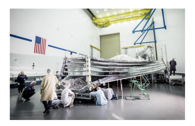
In this photo, engineers and scientists examine the sunshield layers on this full-sized test unit. Credit: Alex Evers/Northrop Grumman Corporation
